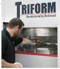
Weldmac's new press joins this 5000-psi sheet-hydroforming press, installed in early 2016, which doesn't require mated tooling or secondary finishing, yet yields complex, net-shaped parts.
