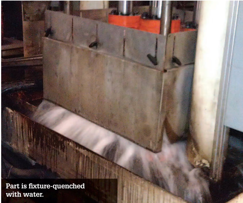
After forming and fixture-quenching, the part is removed from the process.
