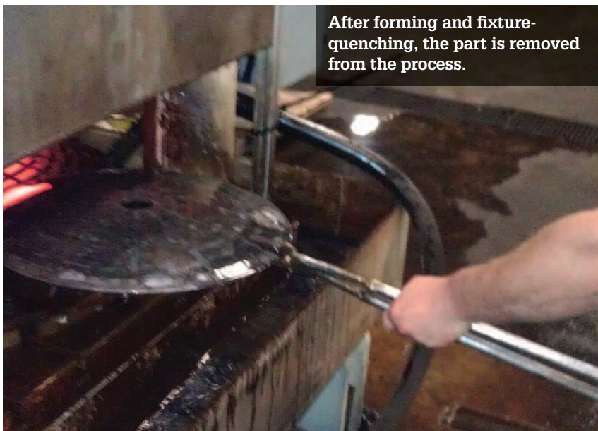
Part is fixture-quenched with water.
