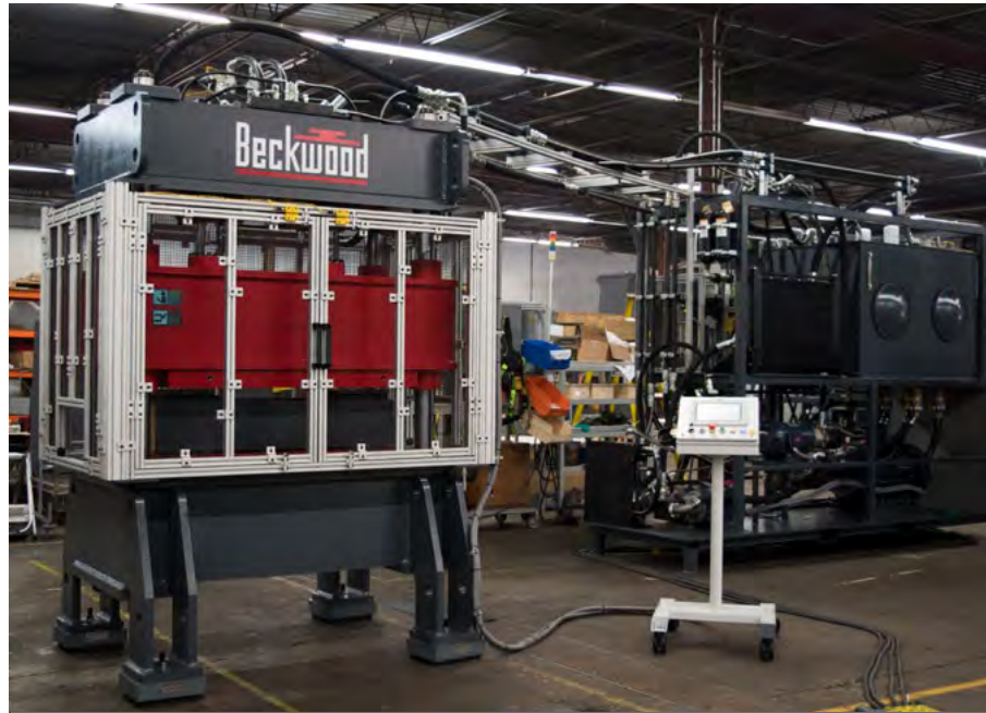
Figure 1 A new hydraulic press, with the ability to deliver 60 cycles per minute or more, meets the speed needs of Dahlstrom Roll Form's roll forming line. Photo courtesy of Beckwood Press Company.
